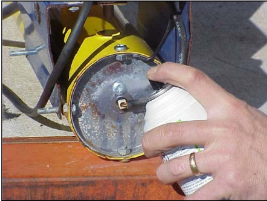
Figure 6. Spray back of electrode and ground wire with silicone conformal coating or similar sealant to prevent corrosion and rust.
