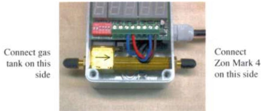
9. Connect the pressure regulator to the gas tank.
