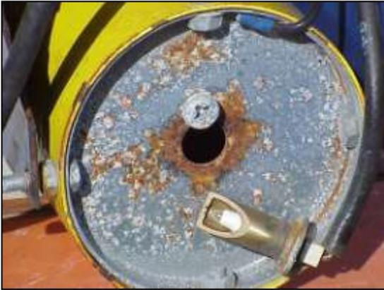
**Figure 1.** Corrosion of rear cover and electrode. Remove electrode from rear cover.
